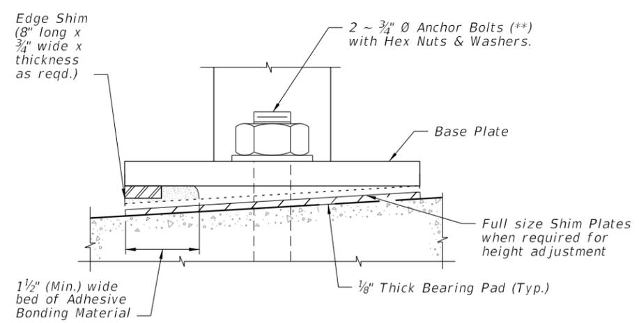
DETAIL "F" (OPTIONAL SHIMMING DETAIL FOR CROSS SLOPE CORRECTION)
