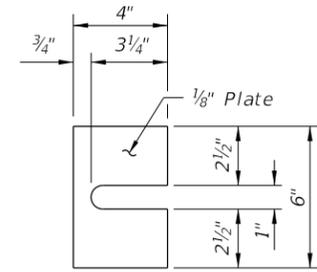
**SHIM PLATE DETAIL (2-Bolt Anchorage)**
